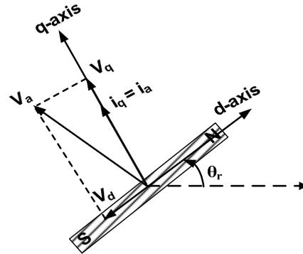
Fig. 2. d-q frame coincides with North Pole of the rotor in case of decoupled vector control.
