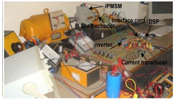
Fig. 7. Experimental set up for IPMSM
