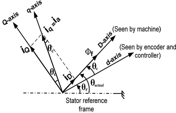
Fig. 3. Phasor diagram showing the relation between current measured d-q frame and actual D-Q frame.
