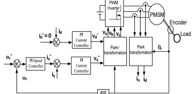
Fig. 1. Decoupled vector control scheme of the PMSM drive.
