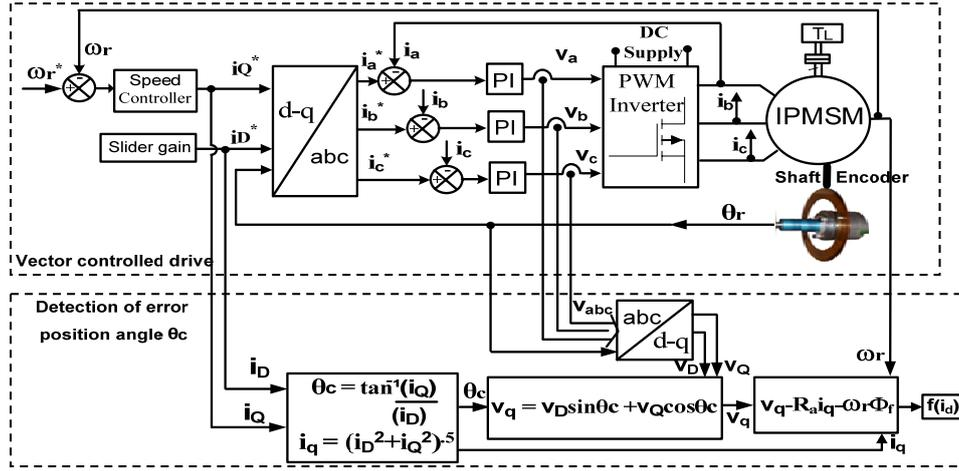
Fig. 4. Block diagram of the novel method to determine the actual rotor position.
