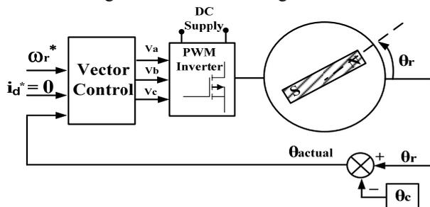
Fig. 6. Experimental diagram of the rotor position detection
