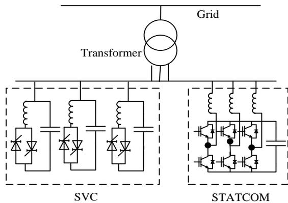
Figure 8: Shunt Compensation using SVC and STATCOM
