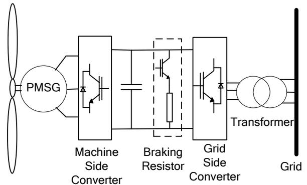
Figure 3: Braking Resistance for PMSG Based Systems
