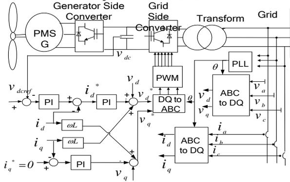
Figure 6: Control of Grid Side Converter
