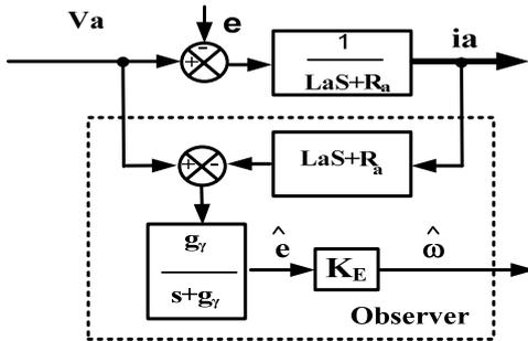
Fig. 1. Equivalent block diagram of the observer for estimation of e.m.f.
