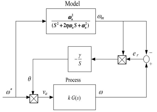
Fig. 2. Block diagram of the MRAS based on the MIT rule
