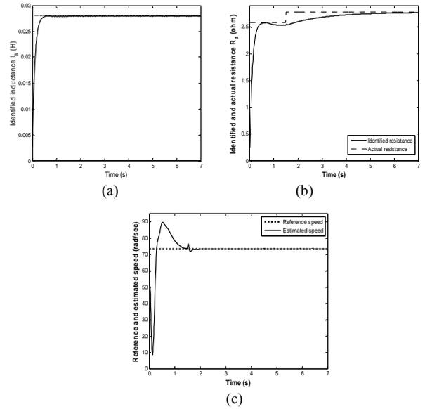
Fig.5. Parameter identification results under heat changes,at rated torque.
