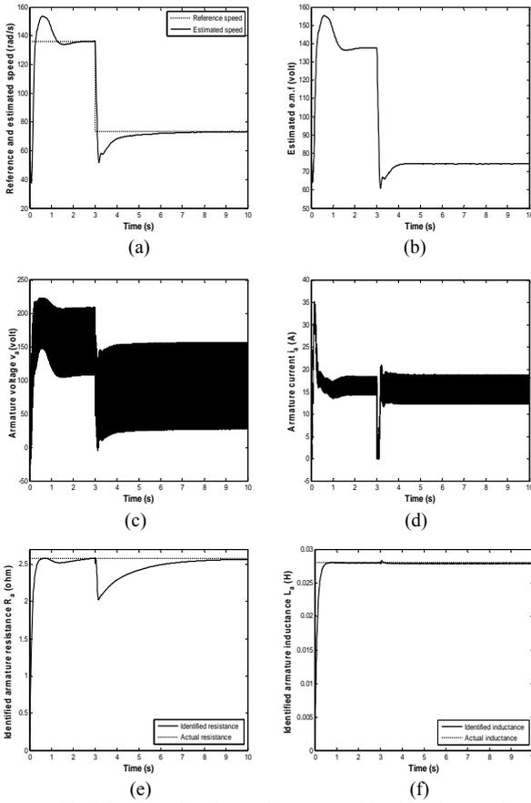
Fig.4.Speed estimation and parameter identification results, at rated load.
