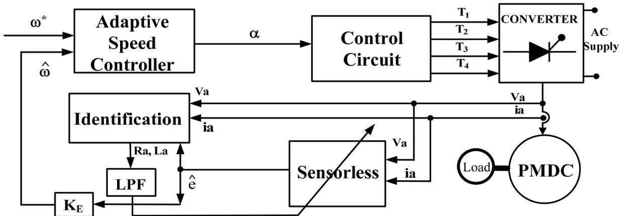
Fig. 3. Block diagram of sensorless control PMDC drive scheme with on-line parameter identification system.
