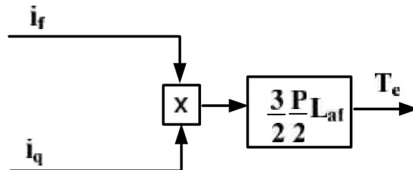
Fig. 2 Torque production-field orientation with constant field excitation.
