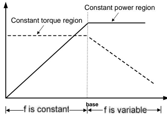
Fig. 4 Constant torque and power region operation.
