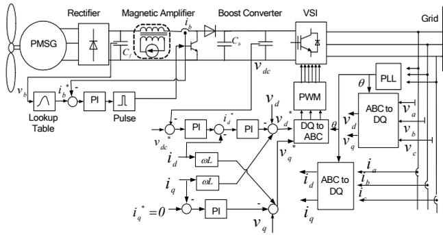
Figure 5: WECS with magnetic amplifier in DC Side
