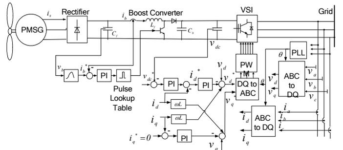
Figure 1: Block diagram for WECS using PMSG
