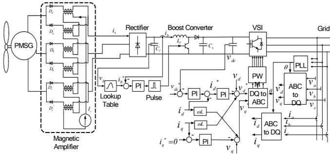
Figure 3: WECS with magnetic amplifier in AC Side
