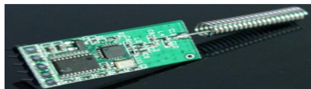
Fig .3. Wireless Module Serial transmitter UART (200M Range-433 Mhz)
