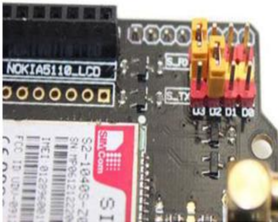
Fig. 11 LCD5100 interface and serial port
