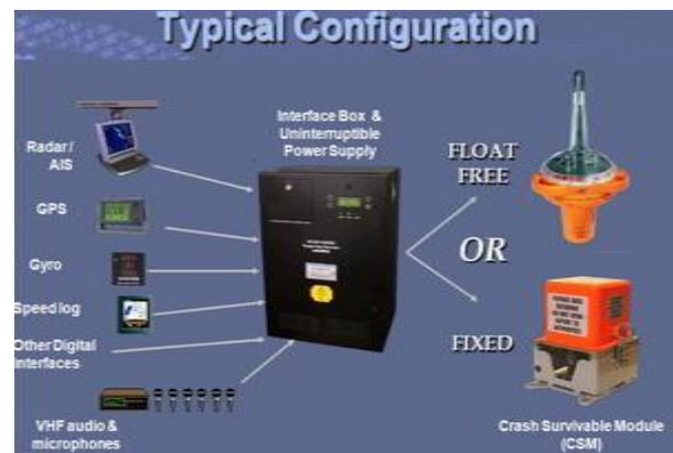
Fig. 2. Typical Configuration for VDR
