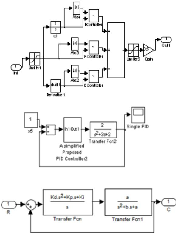
Fig.5 The Proposed PID controller Block Diagram
