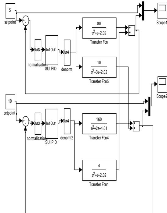
Fig.10 The 2<sup>nd</sup> order Multi input multi output system with SUI PID controller
