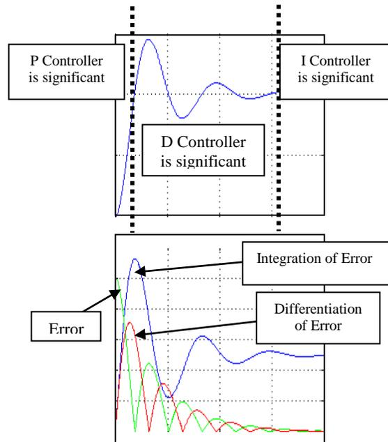
Fig. 4 The system response and the absolute values for error, integration of error and differentiation of error
