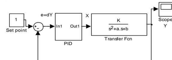
Fig.1 2<sup>nd</sup> order system block diagram
