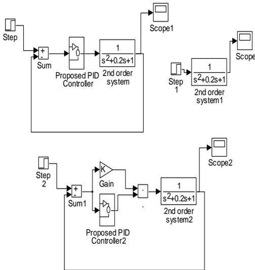
Fig.8 The 2<sup>nd</sup> order system, universal controller and the intelligent PID controller
