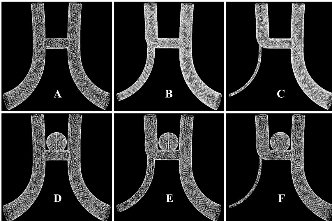
**Fig. 1** Schematic drawing for the unstructured tetrahedral grids representing the six vascular models. **a** and **d** demonstrate the ACOMA geometry with equal A1 arteries (3.5 mm at inflow (A1); 2.5 mm at outflow (A2)) with (**d**) and without aneurysm (**a**). **b** and **e** demonstrate the ACOMA geometry with unequal A1 arteries (50%
