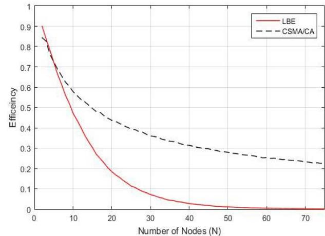
Fig. 7 Efficiency for LBE-based LBT and CSMA/CA with average q value
