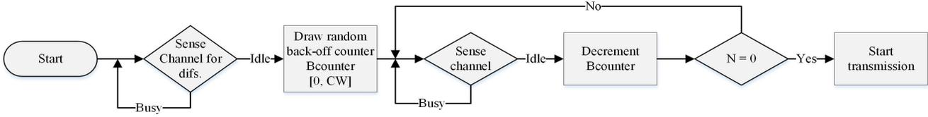
Fig. 3 CSMA/CA process flowchart [12]
