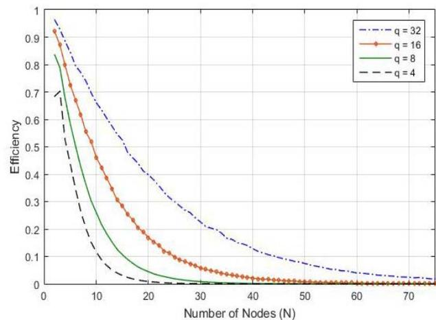
Fig. 5 Efficiency for LBE-based LBT with different  $q$  values
