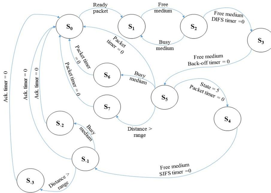
Fig. 4 Proposed CSMA/CA State diagram
