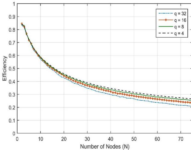
Fig. 6 Efficiency for CSMA/CA with different q values
