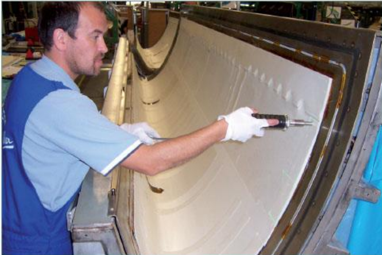
Fig. 10: Ultrasonic welding, A380 J-nose skin
