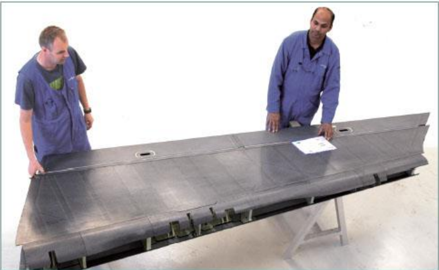
Fig. 3: Welded Gulfstream G650 thermoplastic rudder
