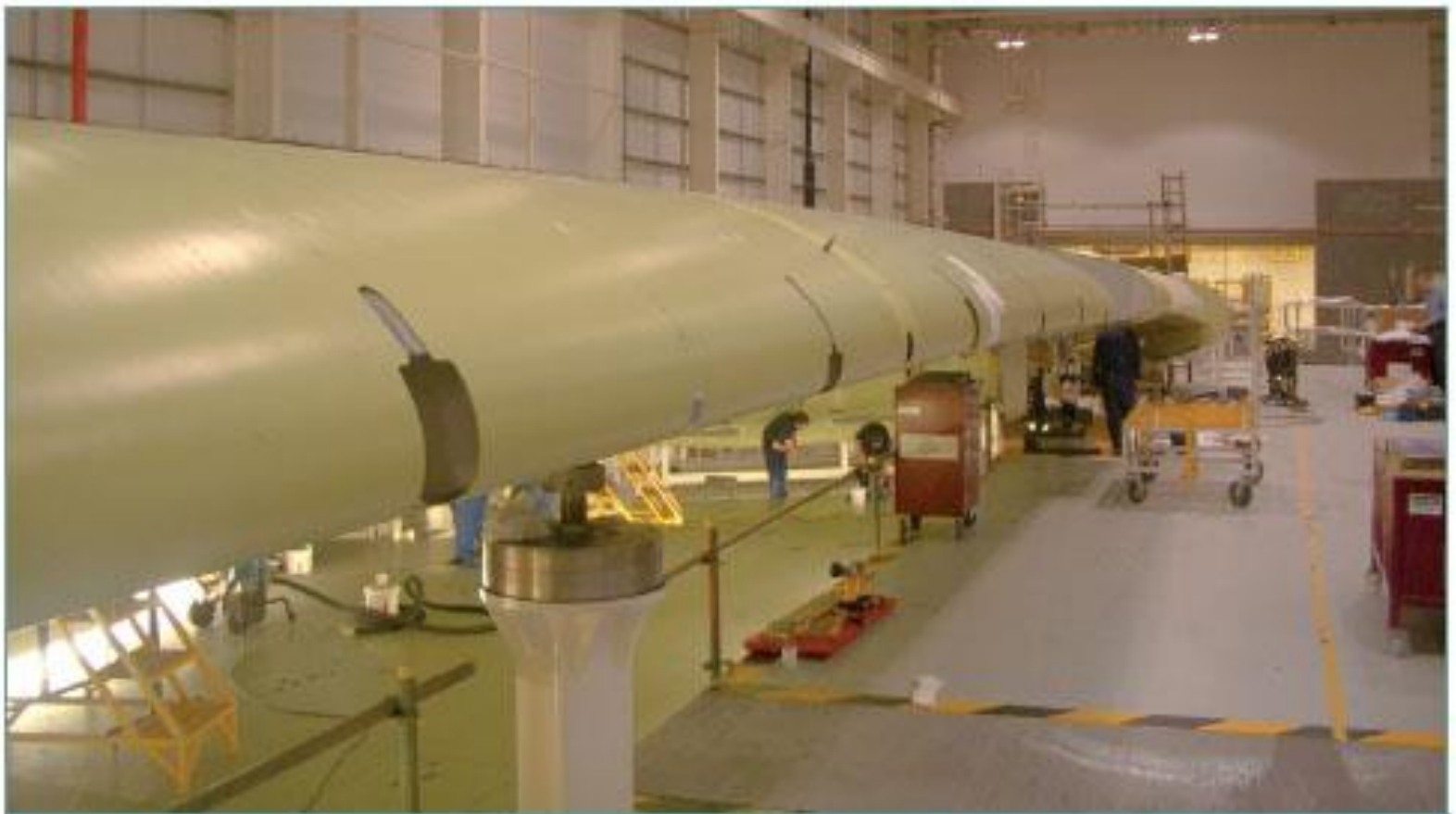
Fig. 1:Welded fixed wing leading edge on an A380 wing (photo courtesy Airbus)
