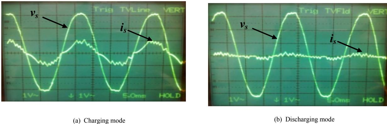
Fig.7. Experimental waveforms of the input supply voltage and current (vs/10)
