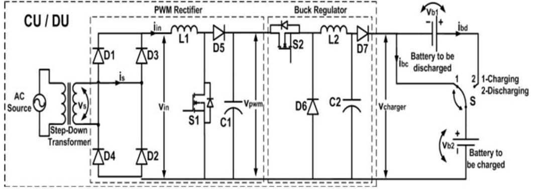
Fig.1. Proposed battery charger / discharger set
