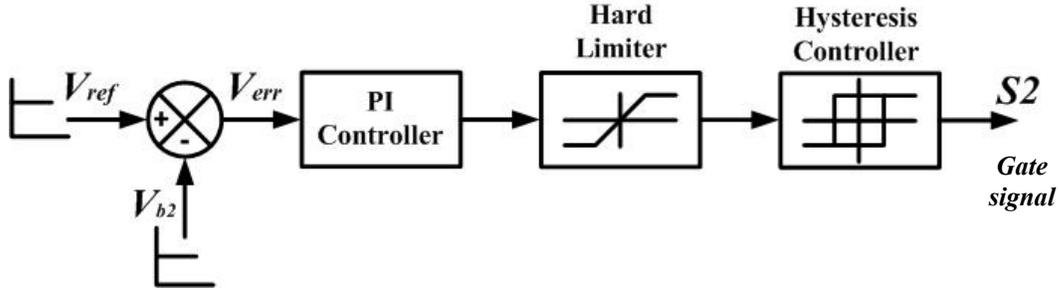
Fig.3. Proposed control loop of the buck regulator
