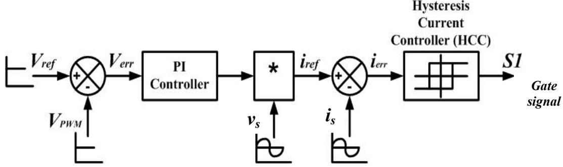
Fig.2. Proposed control loop of the PWM rectifier
