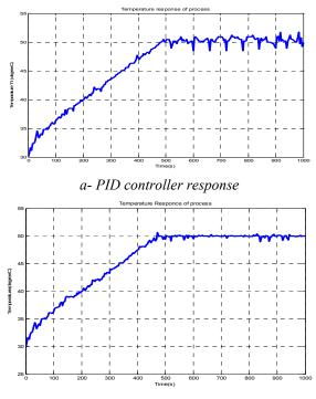
*b- Adaptable PID controller response* Fig. 10. Practical results
