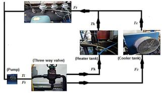
Fig. 1. The temperature process control unit
