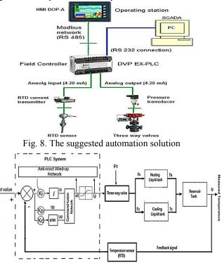
Fig. 9. Overall block diagram of the investigated system
